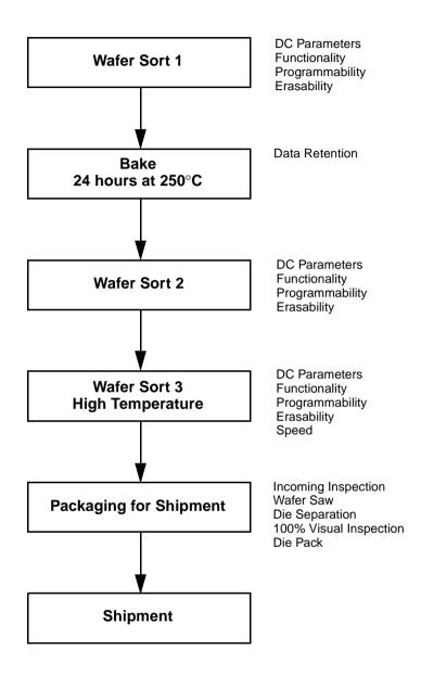
Figure 1. AMD KGD Product Test Flow
